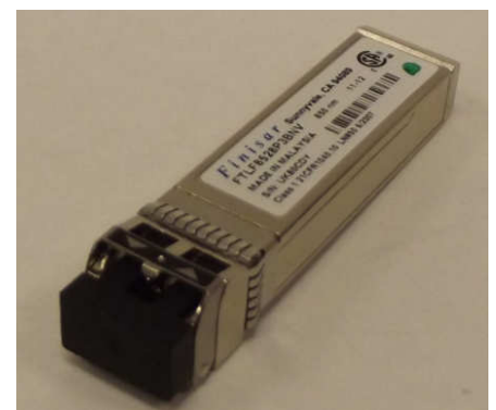
Dust plug in unused SFP+.
