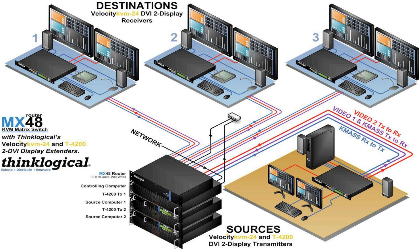
System Design: MX48 Router, KVM Extension provided by VelocityKVM-24 (supports two DVI Displays)
